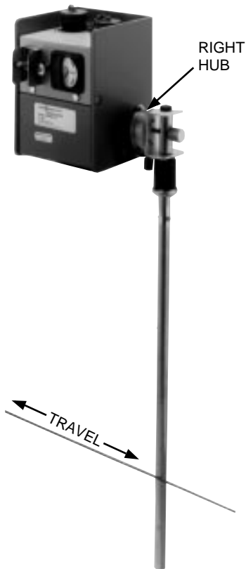
Figure 4. Typical Steering Application. Shaft of the W895A Must Run Parallel to the Stringline.
